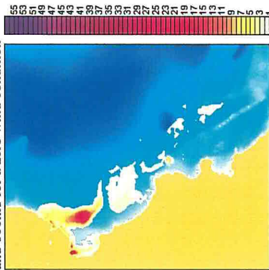
Figure A1.6: Particle distributions after 25, 300, and 600hrs for a zero wind condition
